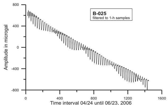
**Fig. 3.** First long interval of the record in the Geodynamic Observatory Moxa from April 24 to June 23, 2006: Note nearly linear drift of about -0.62 mGal per month. Data are filtered to 1-h samples (from Jentzsch [5]).
