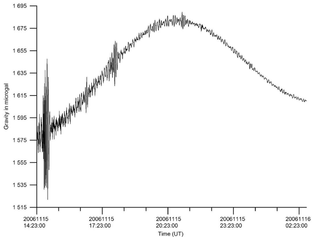
**Fig. 5.** Section of earthquake record (Fig. 4) showing free modes (modified after Jentzsch [5]).
