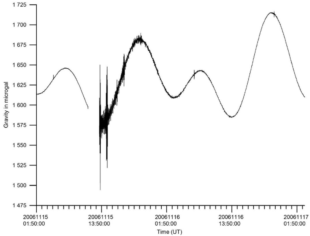
**Fig. 4.** Record Earthquake, Kuril Islands: Nov. 15, 2006, 11:14:17 UTC,  $M_w = 8.3$ . The start of the record is omitted because of the oversaturation due to the large amplitudes (modified after Jentzsch [5]).
