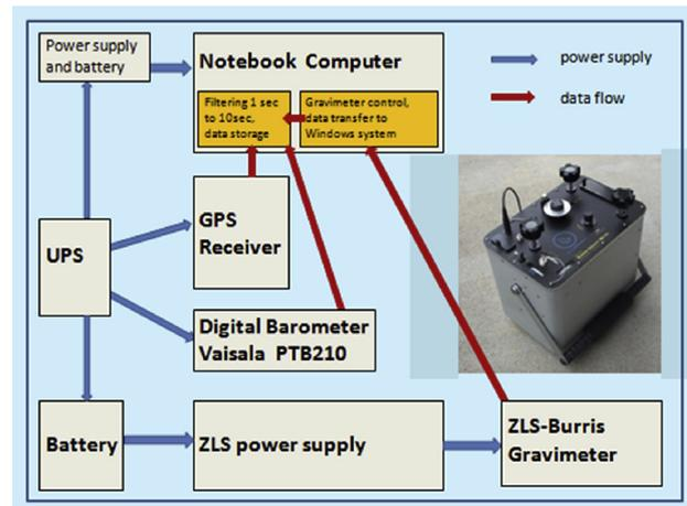
**Fig. 2.** Flow chart of the recording system and components (modified after Jentzsch [5]).
