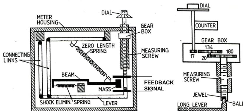
Figure 1. Zero Length Spring and lever system driven by a dial via a gear box: Note sketch of condenser plates to read out the position of the mass and to feed back the voltage necessary to null the beam. (modified after Torge, 1989)
