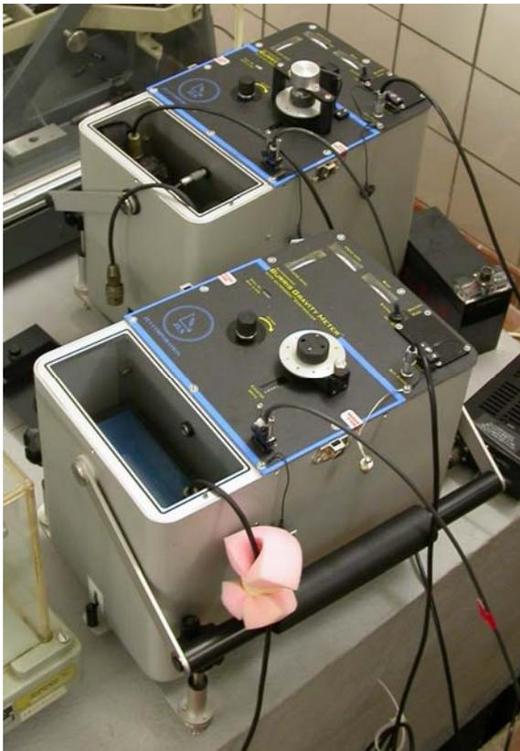
Figure 3. B-025 and B-028 in the Geodynamic Observatory Moxa being tested and equipped with a digital recording system.
