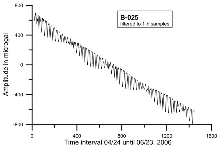
Figure 3. First long interval of the record in the Geodynamic Observatory Moxa from April 24 to June 23, 2006: Note nearly linear drift of about  $-0.62$  mGal per month. Data are filtered to 1-h samples.
