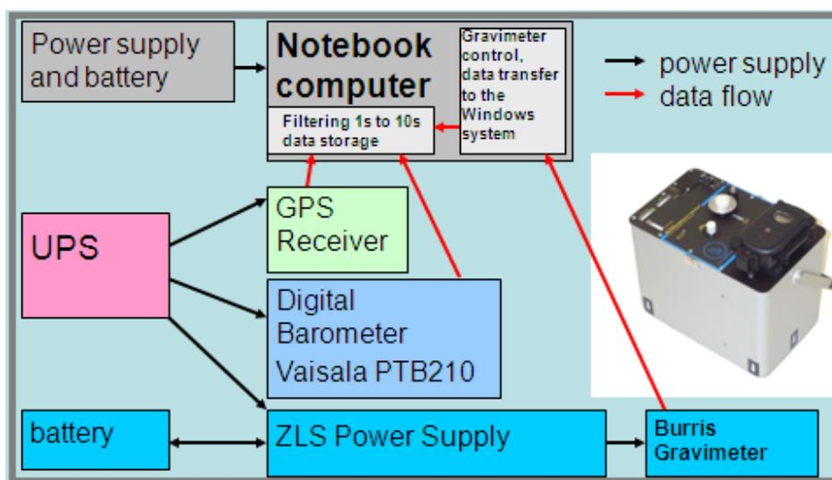
Figure 2. Layout of the recording system consisting of a dual-core notebook computer, the barometer and the GPS time receiver: The computer is used to control the gravimeter and to collect, filter and store the data.
