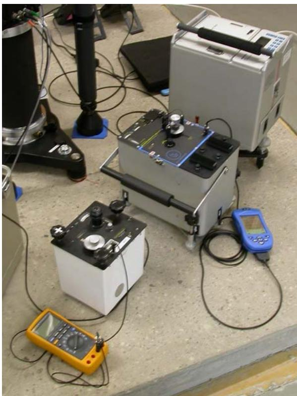
Figure 5. Picture taken during the calibration campaign in Hanover: We can make a visual comparison of the Burris meter with a Scintrex CG3 and a LaCoste & Romberg G-meter equipped with electrostatic feedback system SRW-Hannover.
